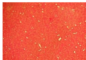
Fig. 1. Photomicrograph of Alpha Tracks in SSNT Detector LR 115 Type II for water sample with 40X objective
