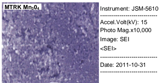
Fig. 3. SEM micrograph of Mn_3O_4 nanoparticles by using hydrothermal method
