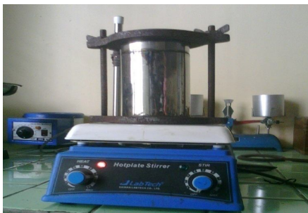
Fig. 1. Teflon-lined stainless steel autoclave (Hydrothermal method)
