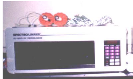
Fig.1. UV cross linker for fixation of DNA to the hybridization nylon membrane.
